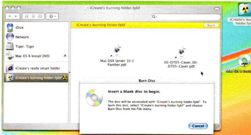
Burning Folders are like regular folders but click on the Burn button and everything in them will write to a CD or DVD
